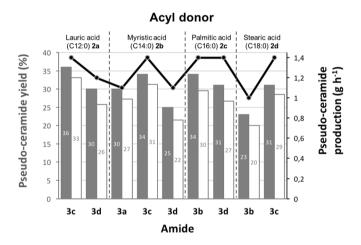
**Fig. 2.** Effect of the nature of the fatty acid used as an acyl donor on the synthesis yield (grey histogram), the overall synthesis yield (blank histogram) and the production rate ( $\bullet$ ) of the 1-*O*,3-*N*-diacyl 3-amino-1,2-propanediol (pseudo-ceramide) produced in step 2, using various amides synthesized in step 1 as acyl acceptors and various fatty acids as acyl donors.
