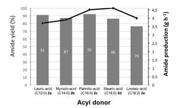
**Fig. 1.** Effect of the nature of the fatty acid used as an acyl donor on the synthesis yield (histogram) and production rate ( $\bullet$ ) of the *N*-acyl 3-amino-1,2-propanediol (amide) produced in step 1, using 3-amino-1,2-propanediol **1** as the acyl acceptor and various fatty acids as acyl donors.
