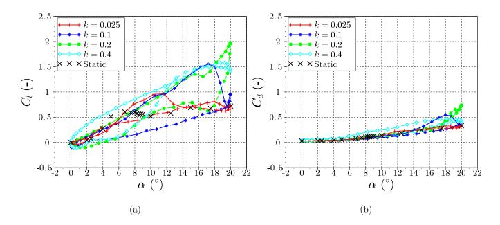
FIG. 6: Phase-averaged lift coefficient (a) and phase-averaged drag coefficient (b) as a function of the airfoil angle of incidence for different reduced frequencies. Airfoil upstroke phases are depicted in plain lines and airfoil downstroke phases are depicted in dashed lines.
