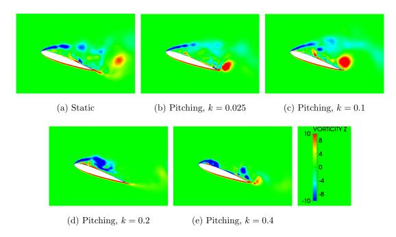
FIG. 11: Contours of non-dimensional spanwise vorticity,  $\omega_Z c/V_0$ , at airfoil midplane for a static airfoil and for airfoils pitching at various reduced frequencies. The angle of incidence is  $\alpha = 19.5^{\circ}$ (upstroke phase).
