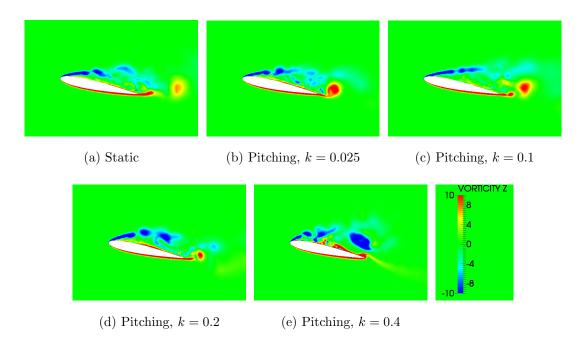
FIG. 13: Contours of non-dimensional spanwise vorticity,  $\omega_Z c/V_0$ , at airfoil midplane for a static airfoil and for airfoils pitching at various reduced frequencies. The angle of incidence is  $\alpha = 11.6^{\circ}$ (downstroke phase).
