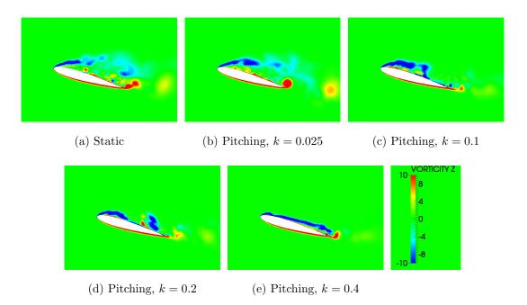
FIG. 10: Contours of non-dimensional spanwise vorticity,  $\omega_Z c/V_0$ , at airfoil midplane for a static airfoil and for airfoils pitching at various reduced frequencies. The angle of incidence is  $\alpha = 15.9^{\circ}$ (upstroke phase).
