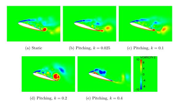
FIG. 12: Contours of non-dimensional spanwise vorticity,  $\omega_Z c/V_0$ , at airfoil midplane for a static airfoil and for airfoils pitching at various reduced frequencies. The angle of incidence is  $\alpha = 18.1^{\circ}$ (downstroke phase).
