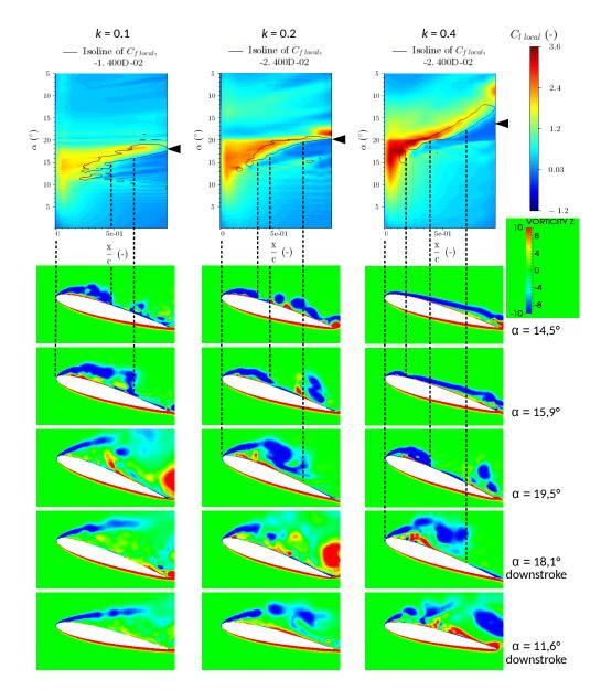
FIG. 16: Top: Local lift coefficient  $C_{l \ local}$  as a function of the dimensionless position on the airfoil suction side and as a function of the incidence with an isovalue line of  $C_{f \ local}$ ; Bottom: non-dimensional spanwise vorticity contours at airfoil midplane for several angles of incidence. Pictures are scaled to observe the LEV influence on the local lift coefficient; Left column:
