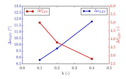
FIG. 18: Angular range  $\Delta \alpha_{LEV}$  and dimensionless time range  $\Delta t^*_{LEV}$  between the moment for which the boundary layer detachment reached the leading edge vicinity and the moment for which the lift and drag coefficients fall as a function of reduced frequency.
