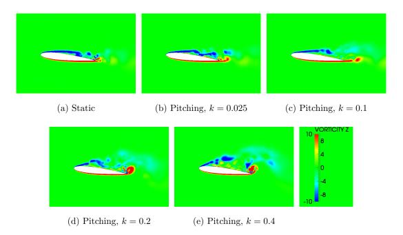
FIG. 14: Contours of non-dimensional spanwise vorticity,  $\omega_Z c/V_0$ , at airfoil midplane for a static airfoil and for airfoils pitching at various reduced frequencies. The angle of incidence is  $\alpha = 6.2^{\circ}$ (downstroke phase).
