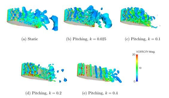
FIG. 5: Q-criterion isosurface colored by non-dimensional vorticity magnitude,  $\omega c/V_0$ , on the airfoil suction side at an incidence  $\alpha \approx 15^{\circ}$ . Static and pitching cases, upstroke part of the motion for pitching cases.
