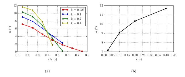
FIG. 15: (a) Position of the boundary layer detachment point as a function of the airfoil angle of incidence, (b) Angle of incidence for which the boundary layer detachment point reached the leading edge vicinity as a function of the reduced frequency.
