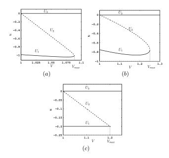
FIG. 3. Bifurcation diagrams of the single block model. Stationary state, u, as a function of the stationary sliding velocity, V, for (a) the regularized generalized Coulomb friction force  $F_{\varepsilon}$  (a = 1,  $\alpha = 0.2$ ,  $\varepsilon = 10^{-4}$ ), (b) the cubic friction force  $F_c$ , and (c) the piecewise-linear friction force  $F_0$  (a = 1,  $\alpha = 0.2$ ). Solid lines represent stable states (denoted  $U_1$  and  $U_3$ ) and dotted lines are for unstable states ( $U_2$ ).
