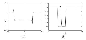
FIG. 7. Plots of velocity waveforms  $u_n(t)$  for the block-spring model. (a) Broad stationary pulse formed after the perturbation of a set of blocks (15 blocks). Parameters are those of Fig. 5(f). (b) Expanding pulse corresponding to a snapshot of the traveling pattern shown in Fig. 4(b) at two different locations (n = 25, n = 50). The initial front propagates at a speed c = 2.45 and the rear front at c = 2 (the moving frame coordinate is  $\xi = n - 2t$ ).
