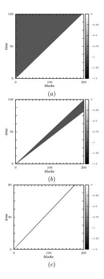
FIG. 4. Numerical simulations of Eq. (8) with the regularized Coulomb friction force  $F_{\varepsilon}$  with the same parameters as in Fig. 3. We display spatiotemporal plots of the velocity variable  $u_n$  of (a) a traveling front (k=0.5 and V=1.01), (b) a broadening pulse (k=1 and V=1.025), and (c) a steadily propagating pulse solution (k=1 and V=1.046). An initial perturbation  $u_0(0)=-10$  is applied on the first block of the chain. Computations are performed for m=0.15.
