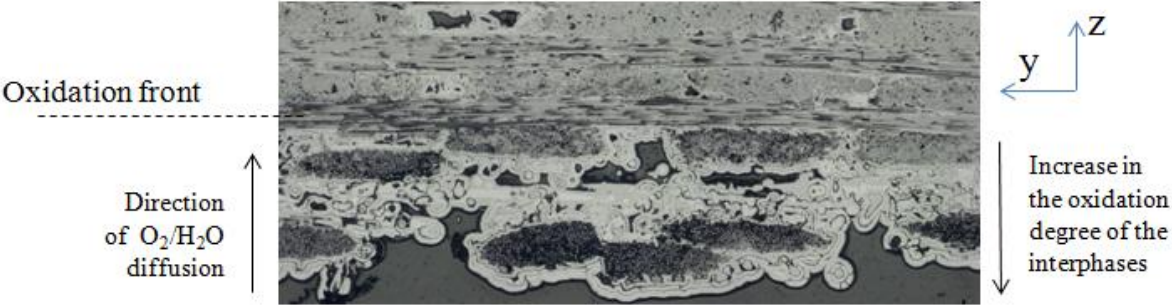
Figure 11- Micrography of a transverse cross-section of sample SM (bottom edge: surface of the sample).
