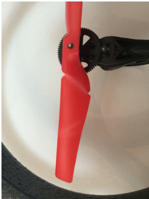
(a) Cut and bended propeller.
