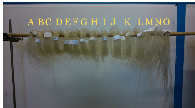
(d) Filaments obtained after extrusion process for use in the OS 3D printer
