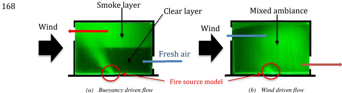
169 *Figure 1: Observation of critical velocity on a reduced scale experiment set up in IUSTI Laboratory, for a simple geometry*
