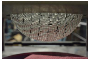
Figure 6- Hemispherical forming experiment on dry fabric
