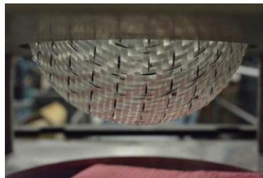
**Figure 6- Hemispherical forming experiment on dry fabric**
