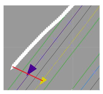
Figure 3. Biased GNSS position and associated matching hypotheses (purple and yellow triangle/line) at the same time index (the GNSS track is displayed in white). The MA-HUL is denoted by the red line, representing the largest distance between the GNSS position and a matching hypothesis. The green lines are the lane markings information from the map.
