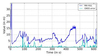
Figure 5. GNSS deviation, computed by comparing with a ground truth (in cyan) and the corresponding computed MA-HUL (in blue).
