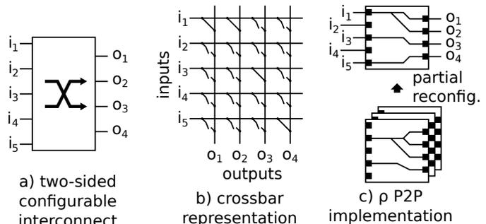
Fig. 1: A 5x4 two-sided interconnect structure and implementations.
