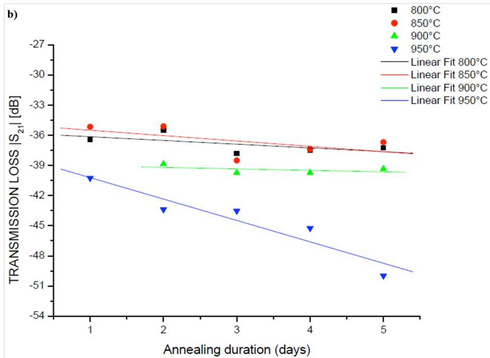
Fig. 11: Transmission losses as function of the annealing duration at different temperatures for the SAW devices based on Ir<sub>0.85</sub>Rh<sub>0.15</sub> (a) and Ir<sub>0.7</sub>Rh<sub>0.3</sub> (b) thin film electrodes.
