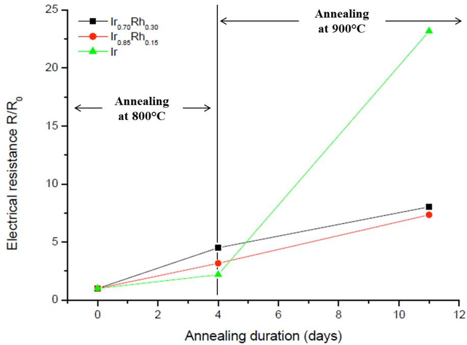
Fig. 7: Relative evolution of the electrical resistance of the Ir,  $\text{Ir}_{0.85}\text{Rh}_{0.15}$  and  $\text{Ir}_{0.7}\text{Rh}_{0.3}$  films during annealing process consisting of 4 days at 800°C, followed by 7 days at 900°C ( $R_0$  being the resistance of the as-deposited films).
