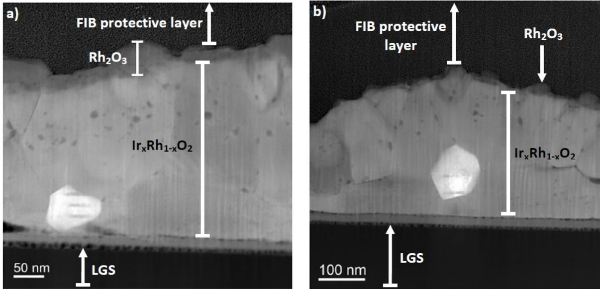
**Fig. 2: Cross-section dark-field TEM image of the  $\text{Ir}_{0.7}\text{Rh}_{0.3}$  (a) and  $\text{Ir}_{0.85}\text{Rh}_{0.15}$  (b) films after a 4 days-annealing period at  $800^\circ\text{C}$  in air.**
