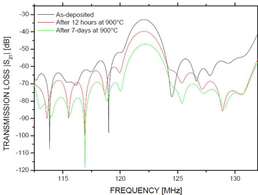
Fig. 12: Frequency response ( $S_{21}$  magnitude) of a SAW delay line based on LGS substrate and 120 nm-thick Ir<sub>70</sub>Rh<sub>30</sub> thin films before and after different annealing periods at 900°C in air.
