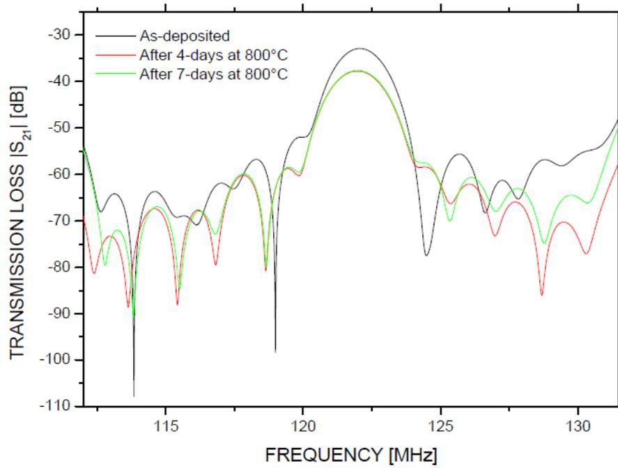
**Fig. 9: Frequency response ( $S_{21}$  magnitude) of a SAW delay line based on LGS substrate and 120 nm-thick  $\text{Ir}_{70}\text{Rh}_{30}$  thin films before and after **different annealing periods** at 800°C in air.**
