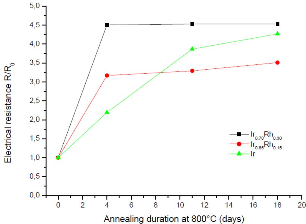
**Fig. 5: Relative evolution of the electrical resistance of the Ir,  $\text{Ir}_{0.85}\text{Rh}_{0.15}$  and  $\text{Ir}_{0.7}\text{Rh}_{0.3}$  films during annealing at 800°C ( $R_0$  being the resistance of the as-deposited films).**
