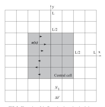
FIG. 2. Illustration of the Brownian dynamics simulation setup. The background velocity  $\mathbf{u}(\mathbf{x})$  vanishes outside the central region, and the particle number  $N_1$  outside in the reservoir region is recorded. The subcells have volume  $\Delta V$ .
