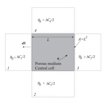
FIG. 4. The porous medium connected to four reservoirs of given constant temperatures and concentration deviations  $\Delta C_i$ . The reservoirs are assumed to be in equilibrium, the central cell is in the steady state, and the concentration deviations are symmetric in the sense that  $\Delta C_{i+2} = -\Delta C_i$ .
