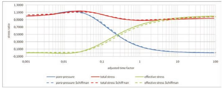
Figure 2. Normalized pore-pressures, total and effective stresses
