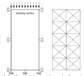
Figure 3. Problem definition and internal cells mesh adopted
