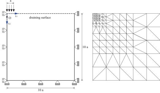
Figure 1. Problem definition and internal cells mesh adopted
