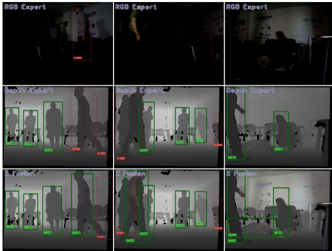
Fig. 10. X-fusion on ONERA.ROOM allows to improve ROIs proposition (left and middle columns) and is even able to detect the unconscious person (right column). However, as for the U-fusion, these strategies suffer from false positive (left column) because they can not remove a detection.
