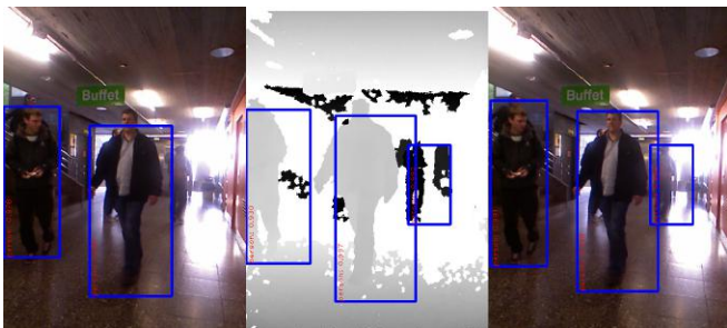
Fig. 4. Examples of predictions with models trained and tested on RGBD People dataset [17], from left to right : RGB expert, depth expert, X-fusion. The depth expert was able to find all the people in the image but the X-fusion propose better bounding box alignments with the ground truth.
