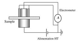
Fig. 2. Principle of current-voltage method.
