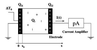
$Q_{i1}$  and  $Q_{i2}$  are the image charges  $Q_i$ : space charge and  $\Delta T_0$ : thermal step.
