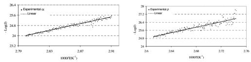
Fig 9 : Variations of -Log (J) = f (1000/T) for the un-heated sample  $E_0$ .
