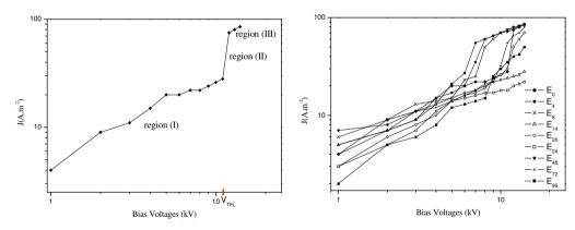
Fig. 12. Current-voltage characteristic of the virgin sample
