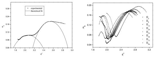
Fig 10. Cole-Cole plots of the dielectric permittivity of the un-heated sample. The two semi circles represent the best fitting of the experimental data.
