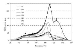
Fig 7. TSDC spectra of un-aged and thermally aged PMMA samples
