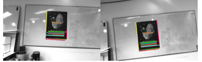
Fig. 2. Successful line matching between the image frame 169 (right) and the reference frame (left). Colorful points in both images are point correspondences used for our line matching algorithm.
