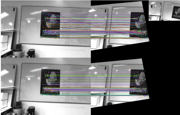
Fig. 1. Matching point correspondences between the warped image frame 264 (warped by the predicted homography) and the reference frame. Poor matching (top) and excellent matching (bottom) before and after applying our outlier removal procedure. Reference frame (left), warped current frame (right), current frame (small image on top right corner).
