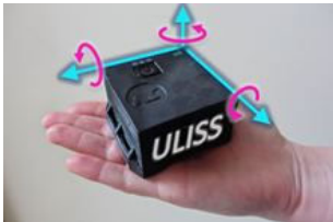
Fig. 5: Ubiquitous Localization Unit with Inertial Sensors and Satellites
