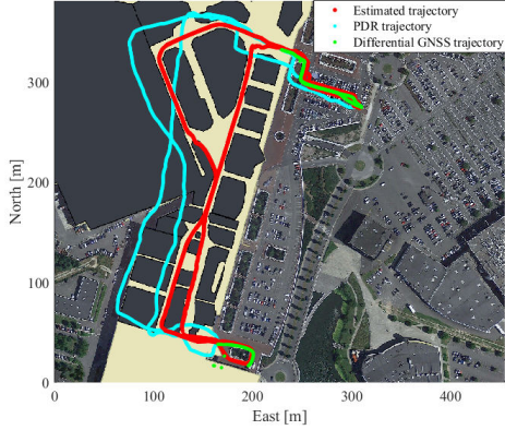
Fig. 7: Estimated trajectory (in red). The Blue trajectory gives the PDR position estimates and the green one gives the reference trajectory (Only Texting)
