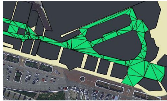
Fig. 1: Walkable zones have been meshed (green polygons). Blank spaces are also walkable but the NavMesh is restricted to our zone of interest. The gray blocks are the stores considered as obstacles.
