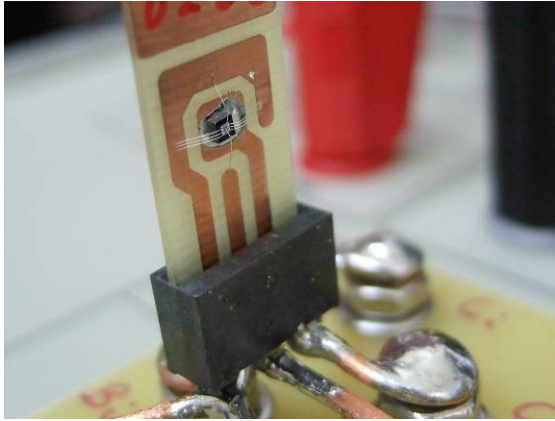
Fig. 5: SiC GTO thyristor with a 3-step JTE attached to a PCB based package and bonded with 50 \mu\text{m} Al wires.
