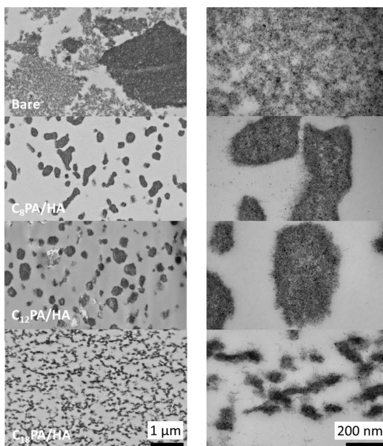
**Figure 3:** TEM pictures of annealed TiO<sub>2</sub>-PMMA nanocomposites at nominal volume fraction  $\Phi = 5\%v$ , in absence of grafting, and with C<sub>8</sub>PA/HA, C<sub>12</sub>PA/HA, and C<sub>18</sub>PA/HA, respectively, for two magnifications.
