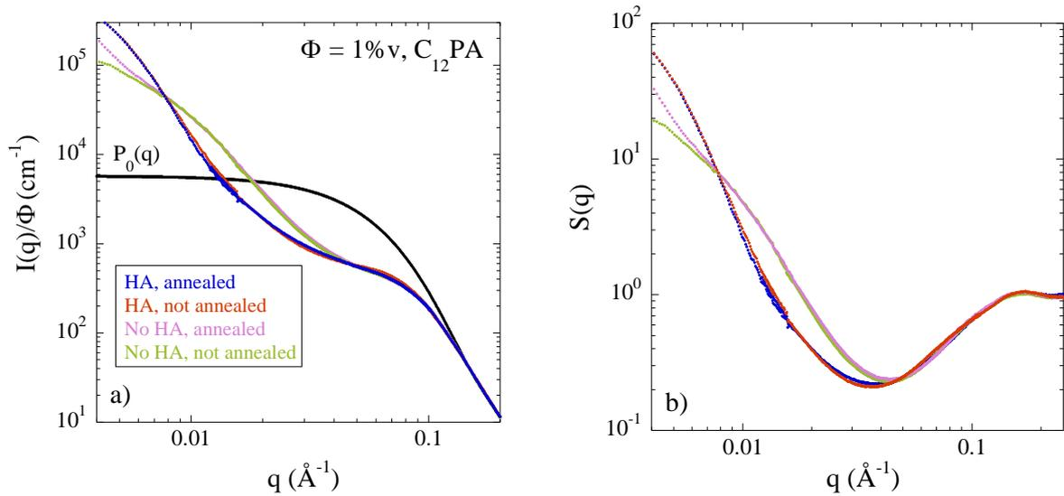
**Figure 4:** **a)** Reduced intensity  $I(q)/\Phi$  of  $\text{TiO}_2$ -PMMA nanocomposites at nominal volume fraction  $\Phi = 1\%v$  grafted with  $\text{C}_{12}\text{PA}$ , or  $\text{C}_{12}\text{PA}/\text{HA}$ , annealed or not, compared to the primary particle form factor. **b)** Corresponding structure factors.
