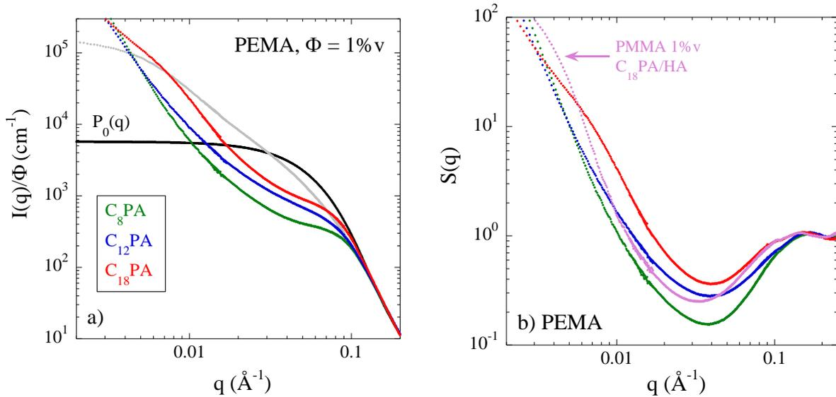
**Figure 5:** (a) Reduced intensity  $I(q)/\Phi$  of TiO<sub>2</sub>-PEMA nanocomposites at nominal volume fraction  $\Phi = 1\% v$ , with surface modification with C<sub>8</sub>PA, C<sub>12</sub>PA, and C<sub>18</sub>PA, respectively, compared to the TiO<sub>2</sub> primary particle form factor  $P_0(q)$ . (b) The apparent structure factor obtained by dividing  $I(q)$  by  $P_0(q)$ . The PMMA/HA nanocomposite structure factor with C<sub>18</sub>PA (annealed) is reproduced for comparison.
