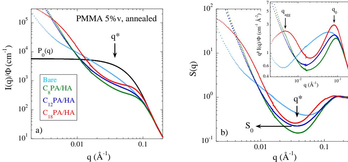
**Figure 2:** **a)** Reduced intensity  $I(q)/\Phi$  of annealed  $\text{TiO}_2$ -PMMA nanocomposites at nominal volume fraction  $\Phi = 5\%$ , in absence of grafting, and with  $\text{C}_8\text{PA/HA}$ ,  $\text{C}_{12}\text{PA/HA}$ , and  $\text{C}_{18}\text{PA/HA}$ , respectively. **b)** Structure factor  $S(q) = I(q)/P_0(q)$  of the same samples. Kratky representations are shown in the inset.
