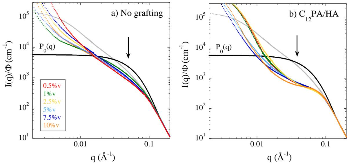
**Figure 1:** Reduced intensity  $I(q)/\Phi$  of annealed  $\text{TiO}_2$ -PMMA nanocomposites for nominal volume fractions  $\Phi$  up to 10% v as indicated in the legend. **(a)** Without grafting, **(b)** with  $\text{C}_{12}\text{PA/HA}$ . The grey curve is the measured NP form factor, and the black one the one of the primary bead  $P_0(q)$  identified with the smaller structural level. The arrow indicates the position of the correlation hole.
