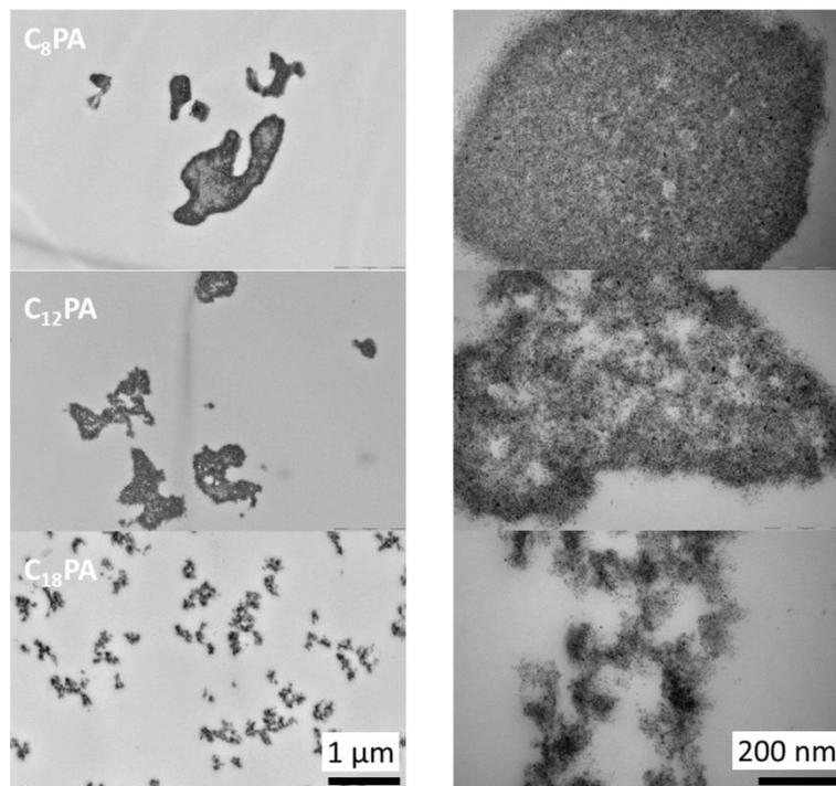
**Figure 6:** TEM pictures of TiO<sub>2</sub>-PEMA nanocomposites at nominal volume fraction  $\Phi = 1\%v$  with C<sub>8</sub>PA, C<sub>12</sub>PA, and C<sub>18</sub>PA, respectively, for two magnifications.
