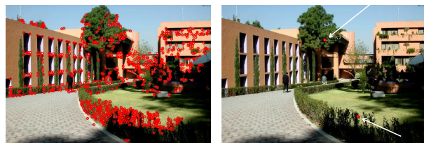
(a) Shi & Tomasi algorithm, threshold = 0.1. (b) Shi & Tomasi algorithm, threshold = 0.8.
