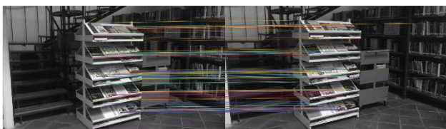
Figure 7: Feature-matching algorithm applied over two consecutive frames from a video sequence.
