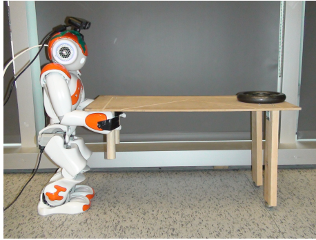
Figure 8: The Nao robot holding the cart-like object and a load
