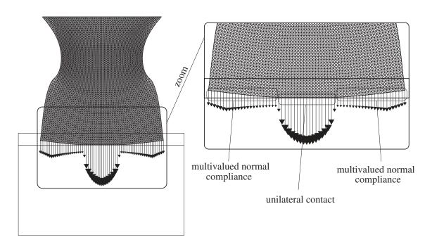
Fig. 5. Deformed meshes and interface forces on  $\Gamma_3$  for Example 3.
