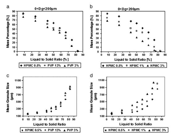
Fig. 6. Evolution of fine particles(a,b) and mean granule size(c,d) for the wet granulation runs with different binders.
