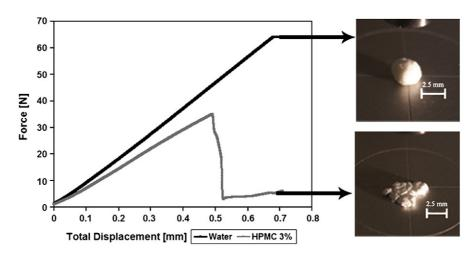
Fig. 10. Typical load displacement curves for large granules obtained from the Diosna HSM using constant impeller tip speed as scale-up rule when using water and HPMC 3% as binders.
