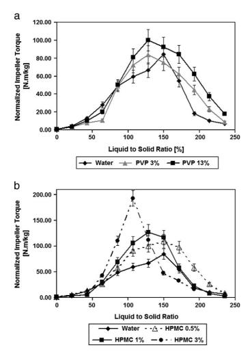
Fig. 3. Mean torque curves on the MTR for the studied binders.
