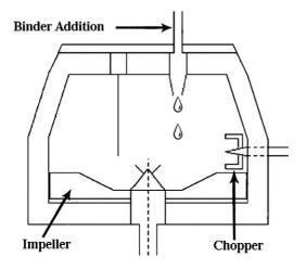
Fig. 2. Diosna P1-6 high shear mixer.
