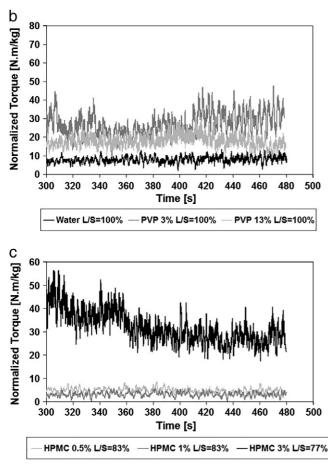
Fig. 7. Typical wet mass consistency evolutions for the studied binders.
