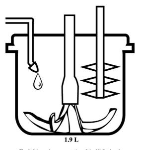
Fig. 1. Schematic representation of the Mi-Pro bowl.
