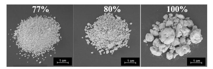
Fig. 5. Final granules obtained in the Mi-Pro 1.9L HSM for different L/S ratios of HPMC 3%.
