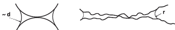
Fig. 6 Liquid bridge of wetted spheres and (left) radius r of curvature of the meniscii for particle with some flatness (right).
