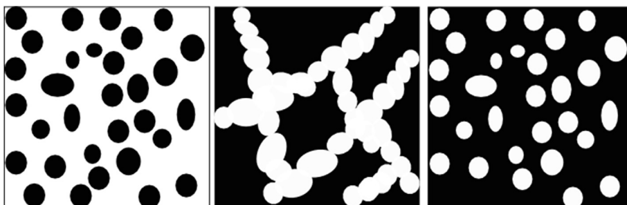
Fig. 1. Scheme presenting different morphological type of phase separation; left to right: particulate, bi-continuous and phase inverted.
