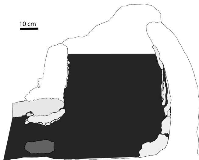
Figure 9: N-S section of Furnace Q. White indicates solid ceramic, light grey more friable ceramic, mid grey fill is stone, and dark grey shading shows the original soil level (with leaf litter on top).
