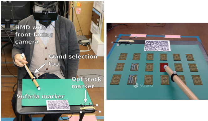
Fig. 3: Left: A participant playing the AR memory card game. Right: First person view of the selection with a wand. NB: the table is also tracked in order to use it as the reference of the 3D space's origin.
