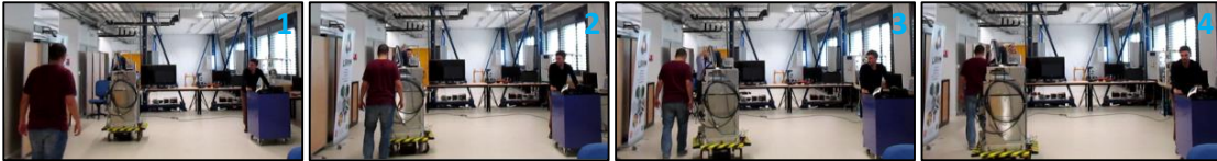
Fig. 15. Real Scenario B: lateral obstacle avoidance while maintaining the blue chariot in sight.
