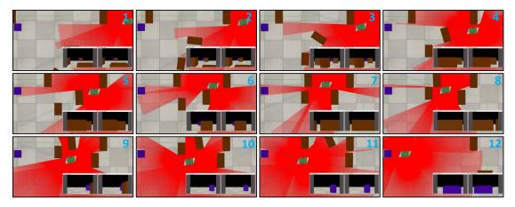
Fig. 6. V-REP Scenario A: the robot (green box), equipped with two cameras (blue cones) and lidar scanners (red lines) navigates towards a static target (blue) while avoiding collisions and dealing with occlusions caused by one static and three moving obstacles (all brown).
