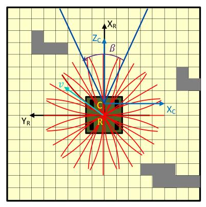
Fig. 1. General definitions. The robot frame  $\mathscr{F}_{\mathscr{R}}$  is shown along with the occupancy grid (yellow), occupied cells (gray), omnidirectional tentacles (red), and visual sensors center (C) with its field of view (blue).
