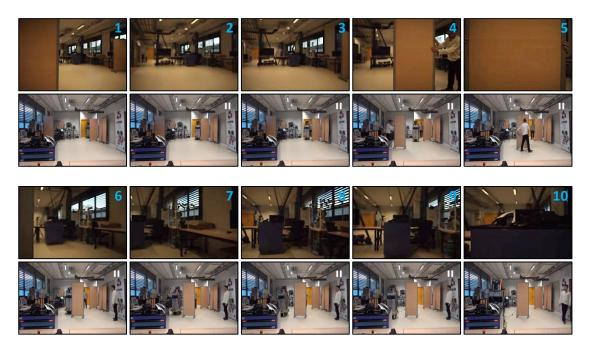
Fig. 11. Real Scenario A: the MPO700 platform navigates safely towards a static blue chariot. Top: images from the left camera, bottom: the MPO700 (grey) avoids two obstacles while dealing with total target occlusion.
