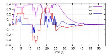
Fig. 7. V-REP Scenario A: robot control inputs (linear velocities  $v_X$  and  $v_Y$  in m/s and angular velocity  $\omega$  in rad/s) during the simulation.
