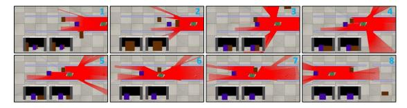
Fig. 10. V-REP Scenario C: the robot follows a moving target in a cluttered corridor with two obstacles (one moving, one static).
