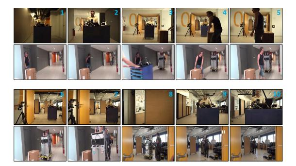
Fig. 15. Real Scenario C: the MPO700 follows a moving target in a cluttered environment, composed first of a corridor and then of a crowded hall.
