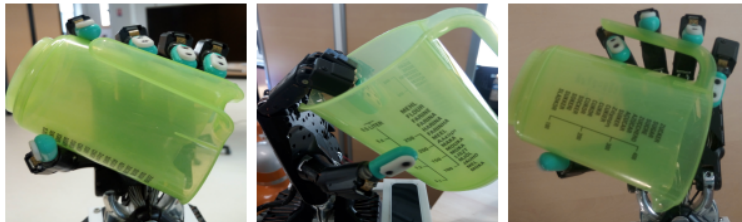
Figure 10: Representative grasps on the "measuring cup" show how different grasps may indicate distinct kinematic features.
