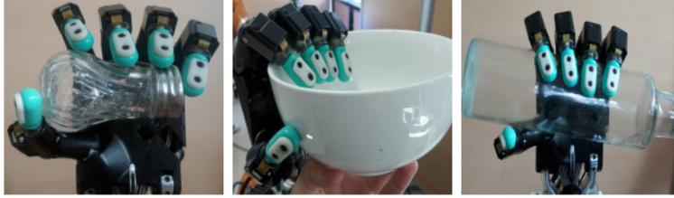
Figure 7: Examples of object grasps by the Shadow Hand.
