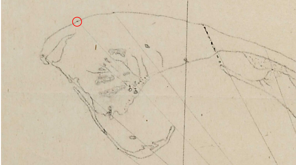
Figure 4: detail of the map on tracing paper (see fig. 2). The red circle is an example of a point of intersection between Thoreau’s radiating straight lines and the coastline of the Cape. Thoreau marked each intersection with his pencil.
