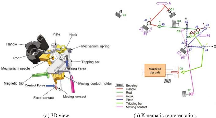
**Fig. 3.** C-60 circuit breaker mechanism - ON position.
