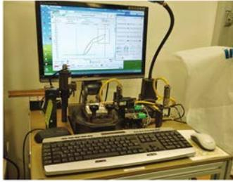
**Fig. 6.** Experimental test bench for contact/tripping force measurement.
