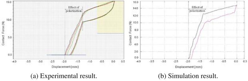
**Fig. 7.** Sample-1: Contact force versus displacement.
