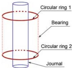
Fig. 4. Revolute joint with clearance  $J_1$ .
