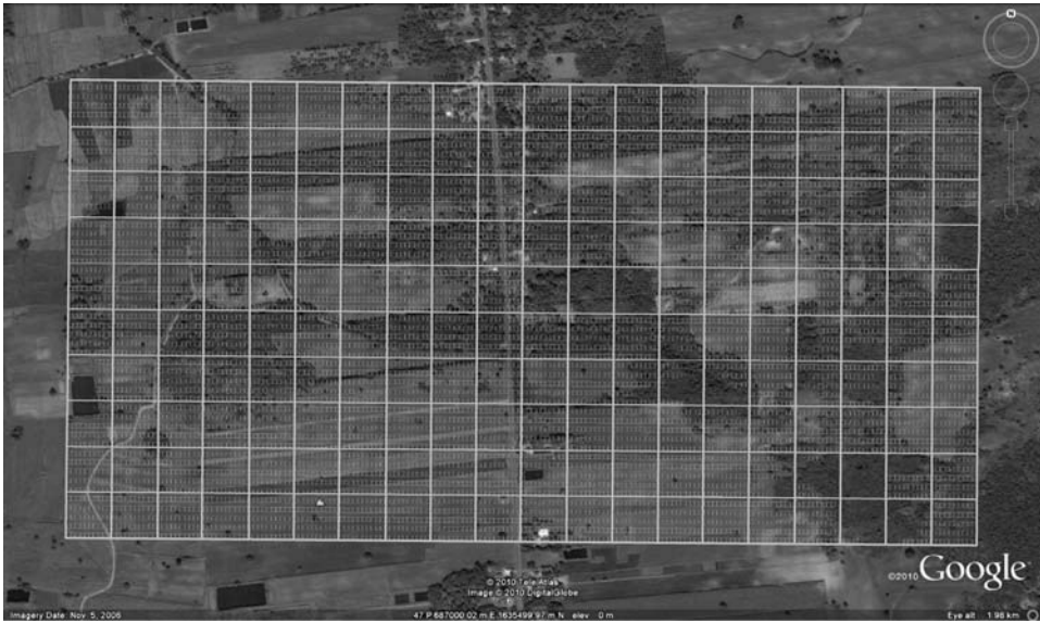
Fig. 3. The division of the Khao Sai On survey area into 1000 m, 100 m, and 10 m units. The southwest corner of the illustrated survey grid is at 686000E, 1635000N (UTM 47N, WGS84). Areas not surveyed by our team have been left unboxed. Underlying satellite imagery courtesy of Google Earth Mapping Services.
