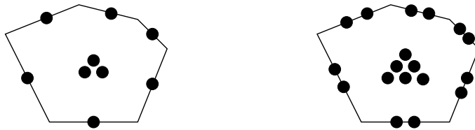
Figure 2: Uncut hexagonal cell. Left: k = 0 ; Right: k = 1 . Each dot attached to a geometric entity (face or cell) symbolizes one degree of freedom (not necessarily a pointwise evaluation).
