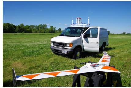
Figure 2. mAEWing1 aircraft: a 10-ft span, low-speed flying wing aircraft (courtesy of the University of Minnesota).
