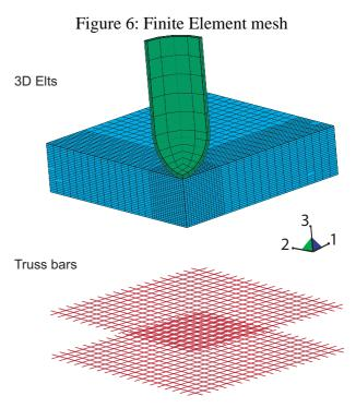
sented by 2300 truss-bars. The impacted area has a refined mesh whereas the other part of the slab has a coarse one.
