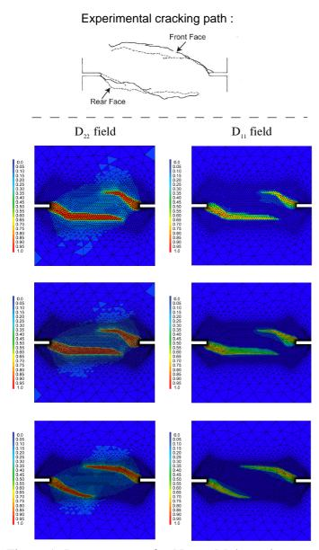
Figure 1: Damage maps for Nooru-Mohamed test at  $U = 3.5 \ 10^{-3} \text{ mm}$ - (a) left column:  $D_{22}$  fields, (b) right column:  $D_{11}$  fields
