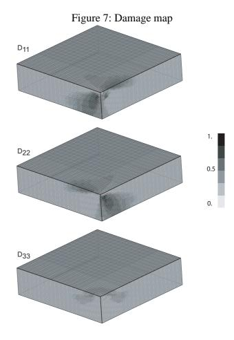
nomenon. In our simulation, damages  $D_{11}$  and  $D_{22}$  are quite large exhibiting a shear rupture of the concrete slab with the apparition of a punch cone as experimentally observed in cases of thin slabs. In the same time, the damage  $D_{33}$  remains small and does not exhibit scabbing.
