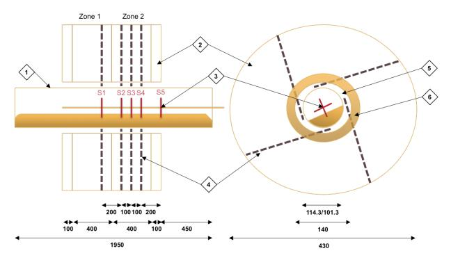
Figure 3: Layout of the experimental apparatus heating zones, longitudinal (left side) and transverse (right side) sections: (1) kiln tube, (2) insulation, (3) measuring rod with N-type thermocouples, (4) outer wall K-type thermocouples, (5) air, (6) heating resistors. The dimensions given in the drawing are in mm.
