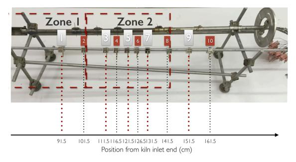
Figure 14: Bed depth measuring rod and position of the stems.
