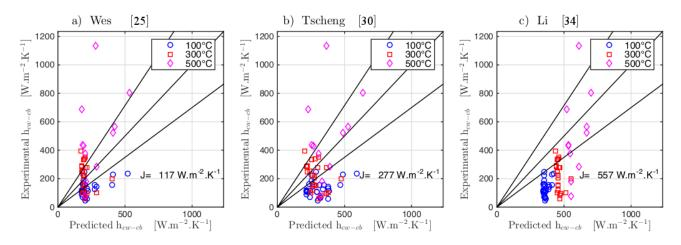
Figure 13: Comparison of the experimental wall-to-solid heat transfer coefficients with the predicted values from the correlations of: a) [25], b) [30], c) [34]. Solid lines are  $\pm 20\%$  margins.
