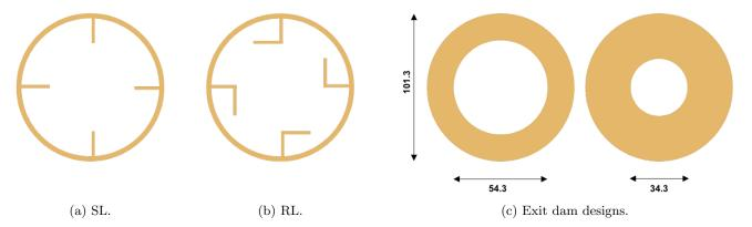
Figure 2: Features equipping the kiln: a) straight lifters (SL), b) rectangular lifters (RL) and c) exit dams.
