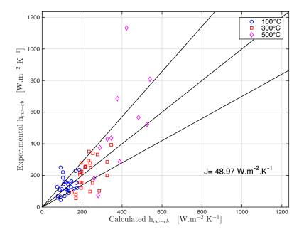
Figure 12: Comparison of experimental wall-to-solid heat transfer coefficients with predictions from Eq.16 using the set of parameters given in Table 4. Solid lines are  $\pm 20\%$  margins. See next section for the definition of the performance criterion J.
