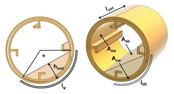
Figure 7: Kiln sections with nomenclature of the heat transfer areas, the bed depth and the filling angle.
