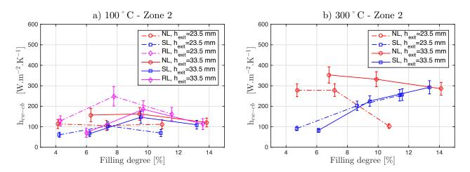
Figure 10: Variation of the wall-to-solid heat transfer coefficient with the filling degree at different setpoint temperatures in zone 2: a) 100°C and b) 300°C, while varying the lifters, the exit dam and the mass flow rate, and operating at a rotational speed of 2 rpm, a kiln slope of 3°.
