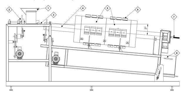
Figure 1: Layout of the experimental apparatus: (1) feed hopper, (2) screw feeder, (3) feed chute, (4) kiln tube, (5) heating system: zones 1 and 2, (6) external thermocouples, (7) measuring rod with thermocouples, (8) storage tank.
