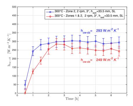
Figure 8: Time variation of the wall-to-solid heat transfer coefficient for both runs represented in Figures 4 and 5.
