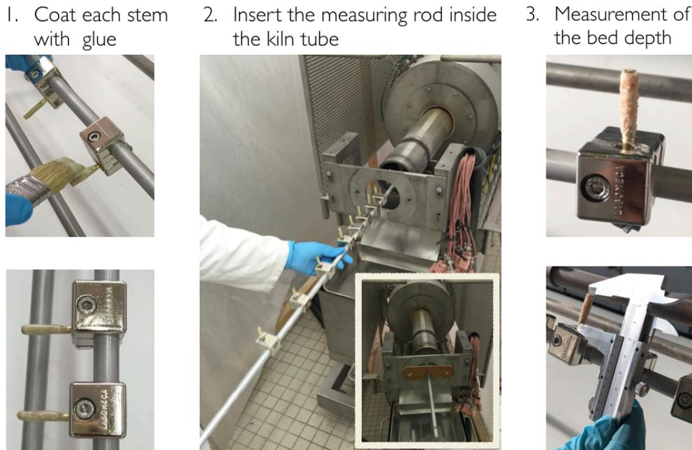
Figure 15: Experimental procedure for the bed depth measurement.
