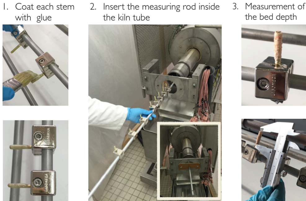
Figure 15: Experimental procedure for the bed depth measurement.
