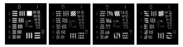
Figure 2: The four raw images used for the myopic SIM reconstruction in the mire test. The first image on the left is the widefield image, and the three other are modulated. The main visible fringes come from the interference between the zero order and the  $\pm 1$  order, with  $k_x/2$  frequency.
