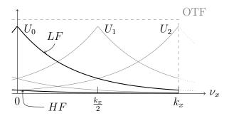
Figure 1: Illustration of amplitude modulation for SIM with zero order. The original spectrum LF is replicated around  $\pm \frac{k_x}{2}$  and  $\pm k_x$ . The OTF removes all frequencies beyond  $\nu_c$ , equal to  $k_x$  in this illustration. The unknown HF part comes from the  $-k_x$  replication while the redundant spectra are in gray.
