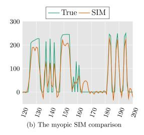
Figure 5: Slice comparison for mire test between the true image, the widefield, and the myopic SIM reconstruction. Figure 5a shows the widefield and the true image. We see that the finer details are no longer visible such as around 140. Figure 5b shows that myopic SIM can estimate these originally lost frequencies.
