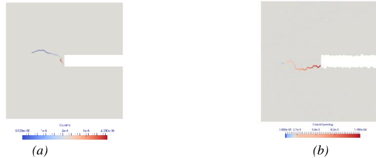
Figure 2. Crack field at the last step of the computation: (a) topological search and crack opening estimation and (b) global/local method.
