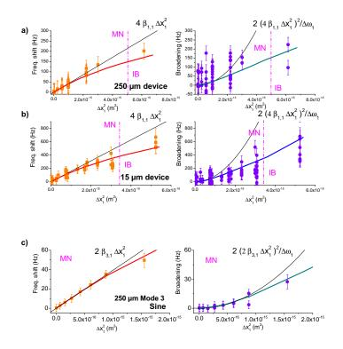
Figure 17: Characteristics for 15  $\mu$ m and 250  $\mu$ m. Same data as Fig. 3 of the paper, for 2 other devices (see tabular 1). a) "self-coupling" on 250  $\mu$ m device. b) "self-coupling" on 15  $\mu$ m device. c) "mode-coupling" on 250  $\mu$ m device. Note that home-made filter and setup characteristics were different, and had to be calibrated following the same procedure as for 300  $\mu$ m devices.
