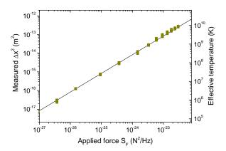
Figure 13: Measured Brownian motion versus applied stochastic force. Measured standard deviation  $\Delta x_1^2$  for sample 300  $\mu$ m-n°2 at 0.84 T with respect to applied force noise (varying the noise current intensity). The line is the theoretical calculation (see text). On the right vertical axis, the motion is converted into effective temperature for mode n = 1.
