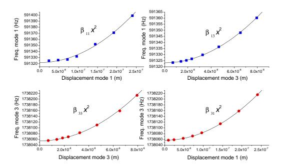
Figure 7: Nonlinear  $\beta_{i,j}$  coefficients. Measurements of the  $\beta_{i,j}$  for device 300  $\mu$ m-n°1. The full lines correspond to quadratic fits enabling to extract the numerical values quoted in the paper.
