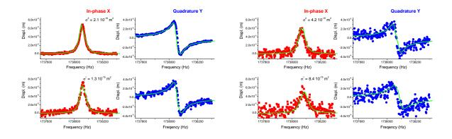
Figure 16: Inter-coupling fits. Data taken on sample 300  $\mu$ m-n°1, measuring mode m = 3 while driving fluctuations on mode n = 1. The applied field is 0.84 T for a force  $F_3^0 = 0.6$  pN; the actual mode 1 position fluctuations are quoted in inset. Calculations (full green line) are explained in the text.
