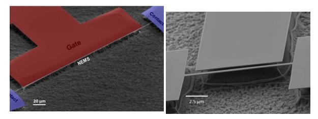
Figure 5: **Devices.** SEM pictures of the devices. Left: 300  $\mu$ m beam (in false colour, the different elements of the device are indicated). Right: 15  $\mu$ m beam. The gates are not used in the present work.
