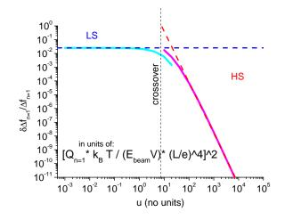
Figure 22: Thermal "dephasing" coefficient vs in-built stress. Calculated sum in the bracket of Eq. (24) for a single family of modes. Here, numerics corresponding to mode n = 1. The overall prefactor is given in inset (see text). The two limits are depicted (low-stress LS and high-stress HS), with their asymptotic behaviors (dashed lines).
