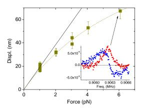
Figure 4: Large sine-wave excitation forces (Color online). Amplitude of the sine-wave response peak as a function of excitation force for mode n = 1 of device 250  $\mu$ m-n°1. Force noise is applied on the same mode n = 1 such that  $\Delta x_1^2 = 2.2 \, 10^{-15} \, \text{m}^2$ . The full line is the linear theory, which clearly does not fit the data (squares and dashed guide). The inset corresponds to the largest drive measured peak.
