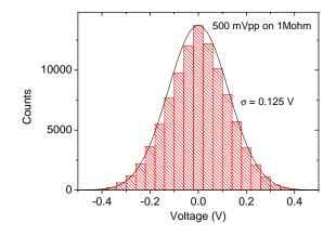
Figure 8: Gaussian noise. Characterization of Gaussian voltage noise. Histogram obtained with a large bandwidth scope; with 1 M $\Omega$  input. The apparatus was the HP34401A, with 0.5 Vpp/50  $\Omega$  settings (delivering thus 1 Vpp on 1 M $\Omega$ ). The line is a Gaussian fit with  $\sigma = 0.125$  V.
