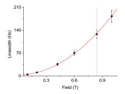
Figure 6: Loading from electric circuit. Linewidth as a function of magnetic field for device 300  $\mu$ m-n°2. The full line is a quadratic fit (see text). The dashed vertical shows were most data have been taken.
