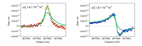
Figure 18: Comparing fits. Data taken on sample 250  $\mu$ m-n°1, measuring mode m = 3 while driving fluctuations on mode n = 1 (X quadrature on the left, and Y on the right). The applied field is 1 T for a force  $F_3^0 = 0.13$  pN; the actual mode n = 1 position fluctuations is quoted in inset. The full green line is the exact theoretical fit, while the dark grey corresponds to the simple average ("inhomogeneous broadening" theory, here peak shifted by about 15 Hz to match data, see text).
