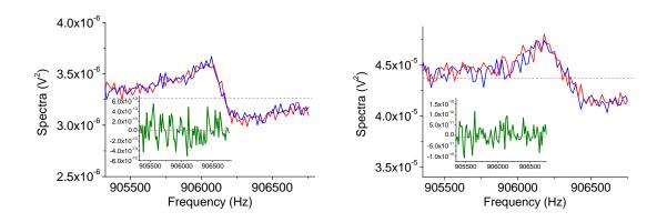
Figure 19: Raw spectra, no sine-wave drive. Raw spectra for mode n=1 measured for small (left,  $\Delta x_1^2 = 2.2 \, 10^{-17} \text{ m}^2$ ) and large (right,  $\Delta x_1^2 = 4.10^{-15} \text{ m}^2$ ) noise levels, with no sine-wave drive. Data from sample 250  $\mu$ m-n°1 taken at 1 T, with X quadrature in red, and Y in blue. The green inset is the cross-correlation spectrum. Acquisition bandwidth 78 Hz.
