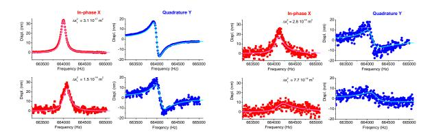
Figure 15: Intra-coupling fits (Color online). In phase (X) and quadrature (Y) components measured for mode n = 1 (first flexure) on sample 300  $\mu$ m-n°2. The sinusoidal force is kept at  $F_1 = 91$  fN, while the standard deviation  $\Delta x_1^2$  (i.e. Brownian motion level) is increased (from top to bottom). Lines are theoretical calculations (see text).
