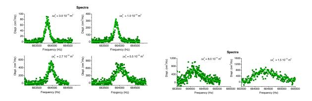
Figure 14: Brownian spectra in non-linear regime (Color online). Measured displacement spectra  $S_X^n(\omega)$  for mode n = 1 (first flexure, no sine-wave drive) on sample 300  $\mu$ m-n°2. The standard deviation  $\Delta x_1^2$  (i.e Brownian motion level) is increased from top-left to bottom-right, and the lineshape distorts from a pure Lorentzian peak to a "Duffing spectrum". Lines are theoretical calculations (see text).
