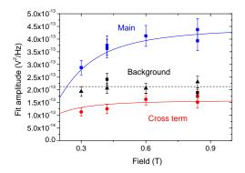
Figure 10: Fit of spectral components vs field. Data taken on sample 300  $\mu$ m-n°2, for a noise drive current of 2.810<sup>-19</sup> A<sup>2</sup>/Hz. Fit parameters are discussed below, and can be related to circuit parameters.
