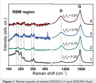
Figure 1: Raman spectra of pristine DWCNTs (1) and DWCNTs fluorinated with  $CF_4$  plasma (2),  $BrF_3$  (3), and  $F_2$  (4).
