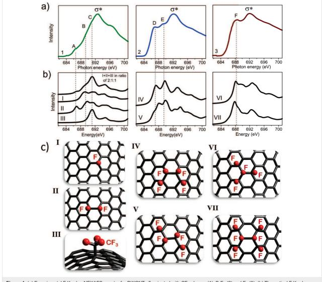
Figure 4: (a) Experimental F K-edge NEXAFS spectra for DWCNTs fluorinated with  $CF_4$  plasma (1),  $BrF_3$  (2) and  $F_2$  (3). (b) Theoretical F K-edge spectra calculated for all F atoms in models (c) distinguished by fluorination pattern. The curve above the theoretical spectra plotted for models I, II and III is their combination in a ratio of 2:1:1.
