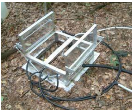
Pic. 1and 2: Example of measuring chamber system (open and closed) used to measure NO & NO 2 fluxes from soil during the experiment at the JRC Ispra forest site.
