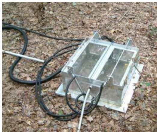
Pic. 1and 2: Example of measuring chamber system (open and closed) used to measure NO & NO 2 fluxes from soil during the experiment at the JRC Ispra forest site.
