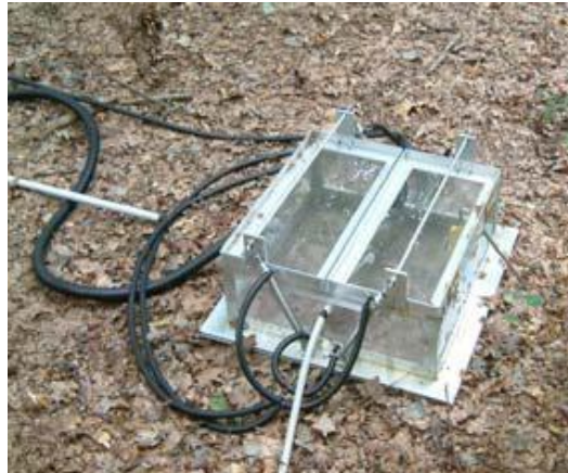
Pic. 1and 2: Example of measuring chamber system (open and closed) used to measure NO & NO 2 fluxes from soil during the experiment at the JRC Ispra forest site.
