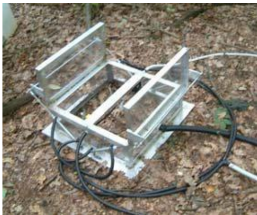
Pic. 1and 2: Example of measuring chamber system (open and closed) used to measure NO & NO 2 fluxes from soil during the experiment at the JRC Ispra forest site.
